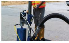
**COMPACT CORE DRILL (OPTION).** The Compact Core Drill allows vacuum excavation to be performed in areas where pavement or asphalt must be removed prior to potholing by cutting a uniform hole into the pavement. Its patented vacuum suction base keeps it securely in place while the hydraulic pump powers the drill. The Compact Core Drill is capable of cutting holes 6 in, 8 in or 10 in (15.2 cm, 20.3 cm or 25.4 cm) in diameter.
