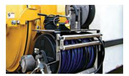
**SEWER JETTER (OPTION).** The J12-30 Sewer Jetter system turns your Vermeer vacuum system into a versatile jetter/vac combination unit. The Sewer Jetter is available on VX75 vacuum systems and is capable of cleaning pipes and culverts up to 12 in (30.5 cm) in diameter. The Sewer Jetter features an electric retract jetter reel and is controlled by a leathered remote.
